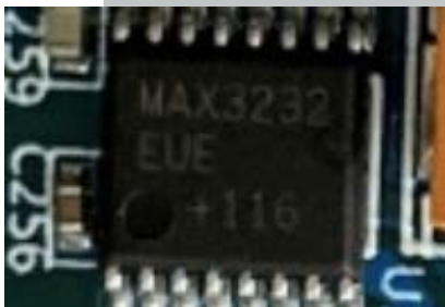
Multichannel RS-232 Line Driver/Receiver manufactured by Maxim Integrated.
