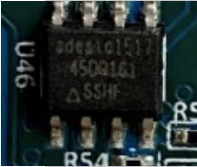
SPI Serial Flash Memory with Dual-I/O and Quad-I/O Support manufactured by Adesto Technologies.
