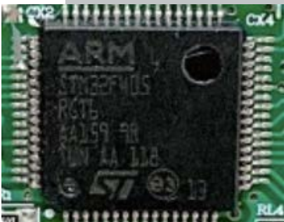
Microcontrollers and linear regulators manufactured by STMicroelectronics.
