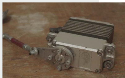
A High Voltage Giant Torque Servo, a form of ultra-precise and efficient electrical motor, manufactured by Hitec USA Group.
