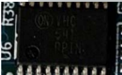
High speed CMOS octal bus buffer manufactured by ON Semiconductor.
