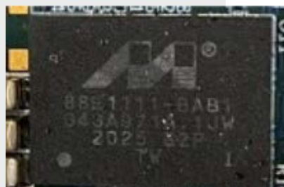
Ethernet transceivers, allowing for point-to-point network and data transfer, manufactured by Marvell Technology. Components bearing the name of Marvell have previously been identified in Russia’s Kalibr cruise missile.
